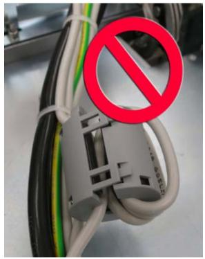
o Ensure the proper number of turns, close the choke, and secure with a cable tie:
