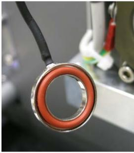
Here is an example of a bad solder joint and ring:
