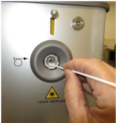
o Continue cleaning the connectors until used swabs are no longer soiled from debris
