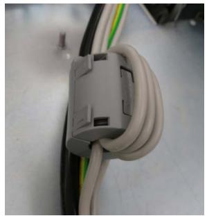
o If the choke has opened due to vibration, and/or there are not three turns through the choke:
