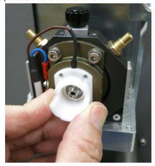
The BROWN wire is soldered to the chrome ring. This solder joint can crack. Carefully inspect this connection front and back to ensure a good joint. If you must re-solder, REMOVE THE O-RING FIRST!! The wire actually enters a very small hole in the ring. It will be necessary to remove the solder from the hole and reflow fresh solder if the connection is bad. Do not flow an excessive amount of solder onto the joint, space is limited on re-assembly:
