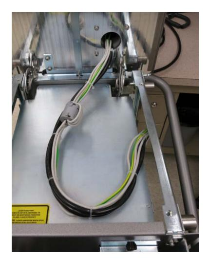
The RF choke seen here in the cable should be closed, and have three turns of the gray wire passing through it.
