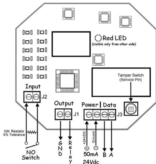
The Gen-2 IR Location Reader has a Service Pin/Tamper Switch that generates service messages when pressed to aid device registration. The Service Pin/Tamper Switch is also used to indicate attempts to remove the device's cover after the device has been enrolled in EIRIS.
