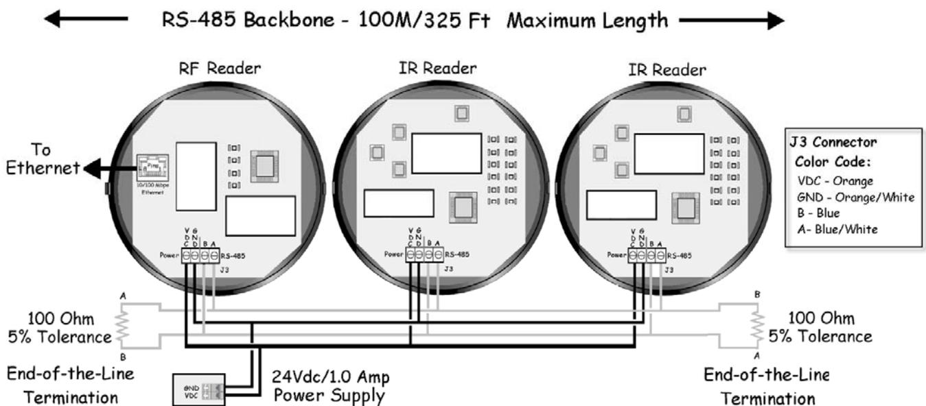
**Recommended Cable Type:** CAT5 Stranded (4x2x26AWG)
