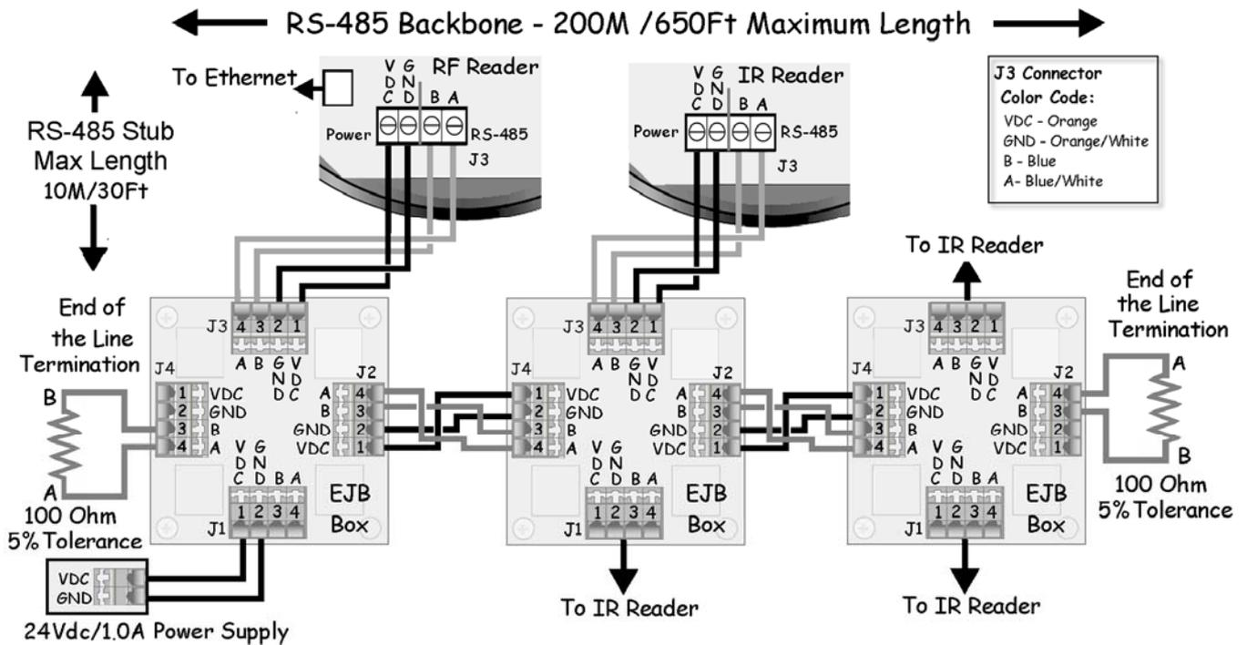
**Recommended Cable Type:** CAT5 Stranded (4x2x26AWG)
