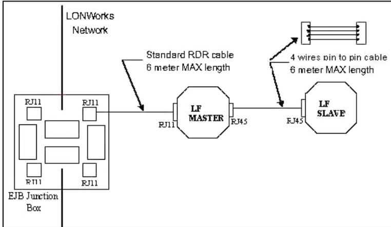
When the Master LF Exciter (from hardware Version C, Revision A-1) senses that the Slave has been disconnected, the B1 bit on the RF supervision transmission is set to Down.
