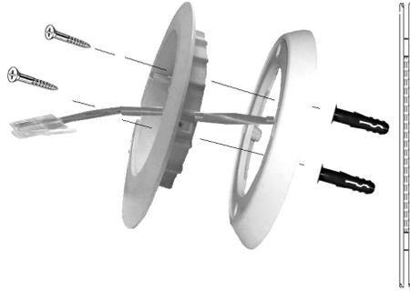
6. Screw the base to the wall or ceiling using the 2 supplied screws. Ensure that the screw heads are recessed inside the screw holes. If not the LF Exciter will not close properly and damage may occur.
