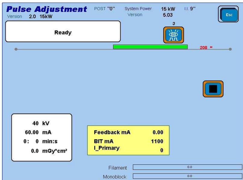
As the calibration ends, wait for 90 seconds before performing the other adjustments (see NOTE in step 3).
