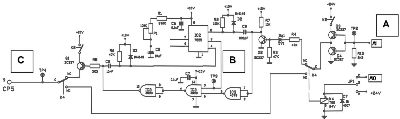
The signal "A" is the X-ray order coming from the microprocessor and defines the X-ray emission time.
