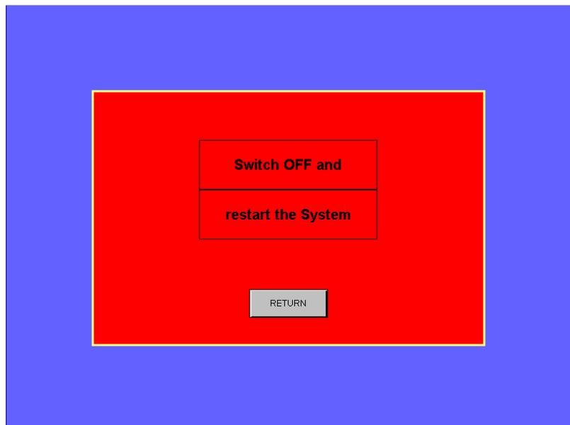
Now the default data are loaded on the system, which means you have to do a full calibration and configure all the system settings again.
