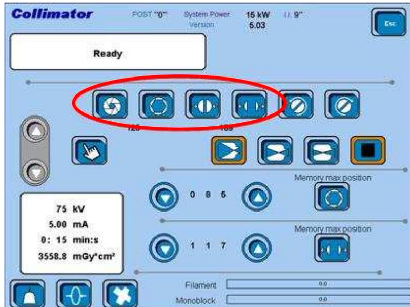
**Step 4 -** Now release the RX switch and read the two values circled below.
