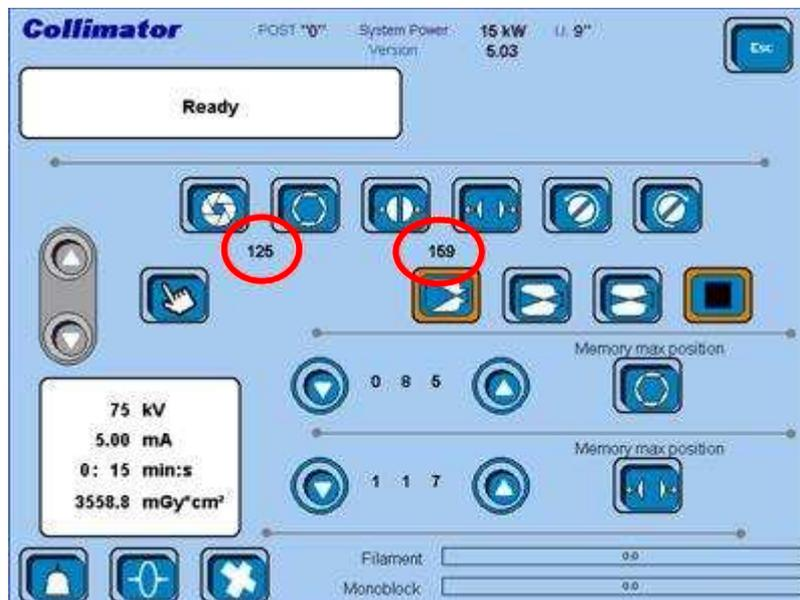
**Step 5 -** Adjust the values circled in the figure below by using the arrow keys.
