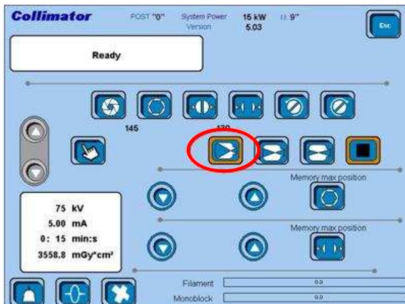
**Step 3 -** Then press the RX switch to make an RX exposition. While the RX button is pressed, use the switches circled in the figure below to set the diaphragms opening.
