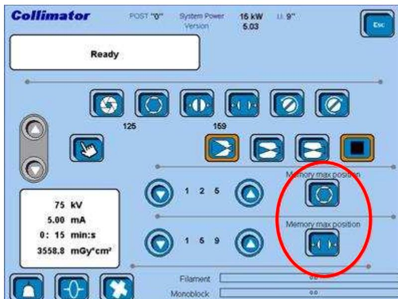
**Step 7 -** To end the collimator calibration you need to repeat this whole procedure for the I.I. zoom 1 and zoom 2.
