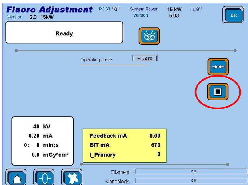
**Step 6 -** You still miss the two calibration for the Isowatt curve; so restart the system, press the button for the selection of the Isowatt curve in the Service page, then restart the system again.
