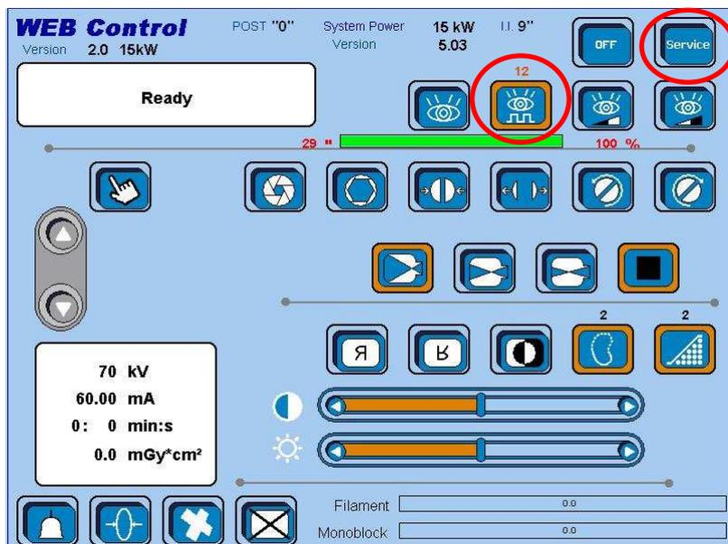
**Step 2 -** You have to do seven calibrations for the pulse mode: three for the large focus and four for the small focus. Select one of the four buttons at the bottom of the screen; here we choose the large focus at 120 mA, but only as an example.
