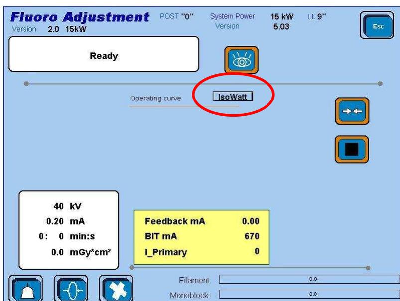
**Step 8 -** At last, select the small focus again, press the two matching arrows button and do the fourth calibration. Restart the system.
