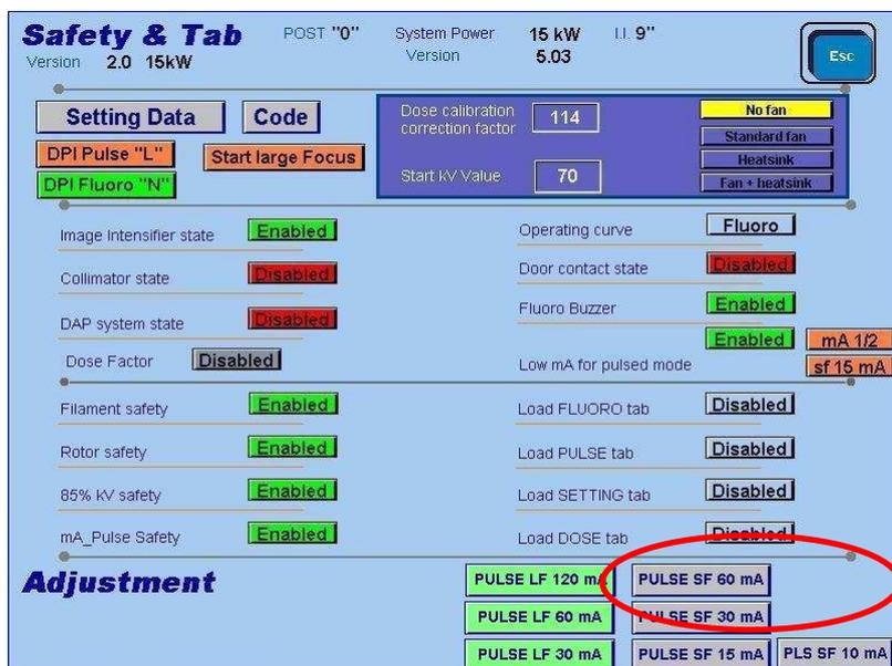
**Step 7 -** Now you are in the Small Focus – 60 mA Pulse calibration page. If the wait time has ended, press the RX button and keep it pressed to do the third calibration.
