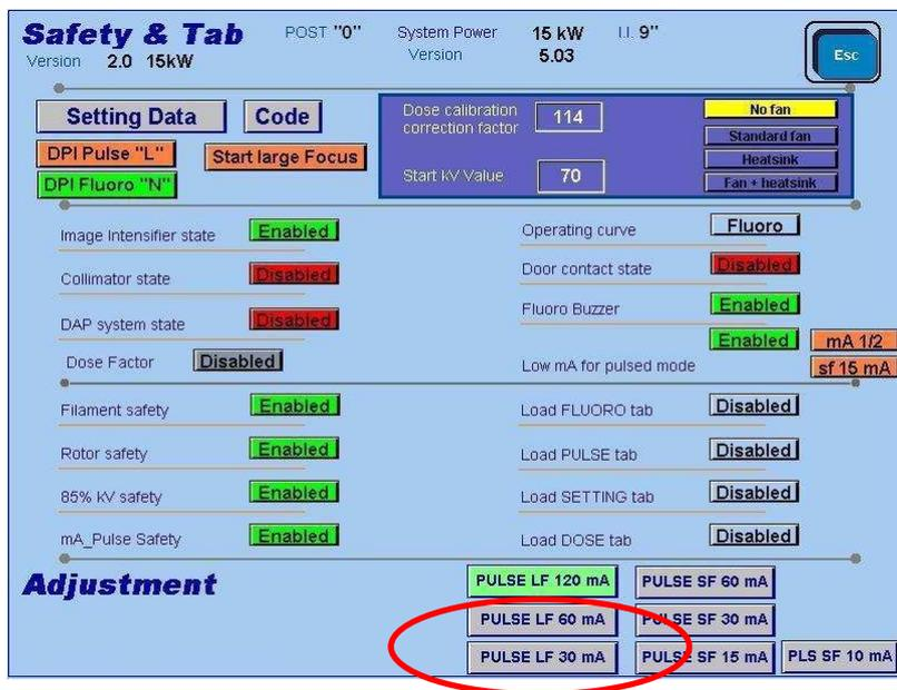
**Step 5 -** Now you are in the Large Focus – 60 mA Pulse calibration page. If the wait time has ended, press the RX button and keep it pressed to do the calibration.
