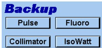
It is recommended to use the Backup function after any calibration. Pressing the buttons on the left allows to save, through four separate files, the data of Pulse, Fluoro curve, Isowatt curve, and Collimator adjustments.
