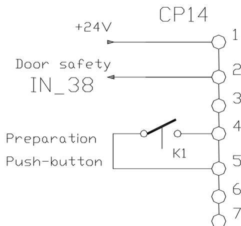
On CP14 connector, pin 4 and 5, there is at disposal a “clean” contact of K1 relay. This contact is closed by radiographic preparation command executed by the remote foot-switch.
