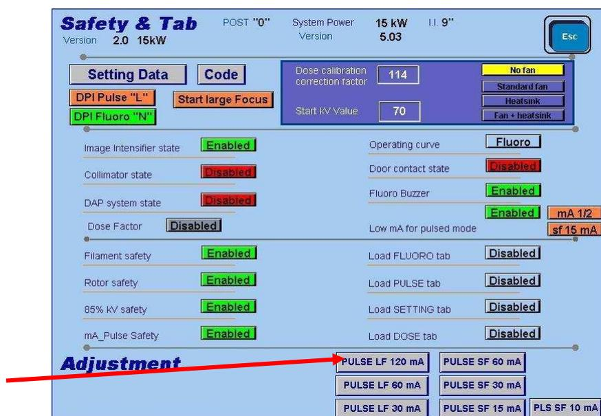
**Step 3 -** Now you are in the Large Focus – 120 mA Pulse calibration page. Just press the RX button and keep it pressed to do the calibration.
