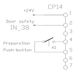
On CP14 connector always, pin 4 and 5, it is at disposal a "clean" contact of K1 relay. This contact is closed by radiographic preparation command execute by remote foot-lever.
