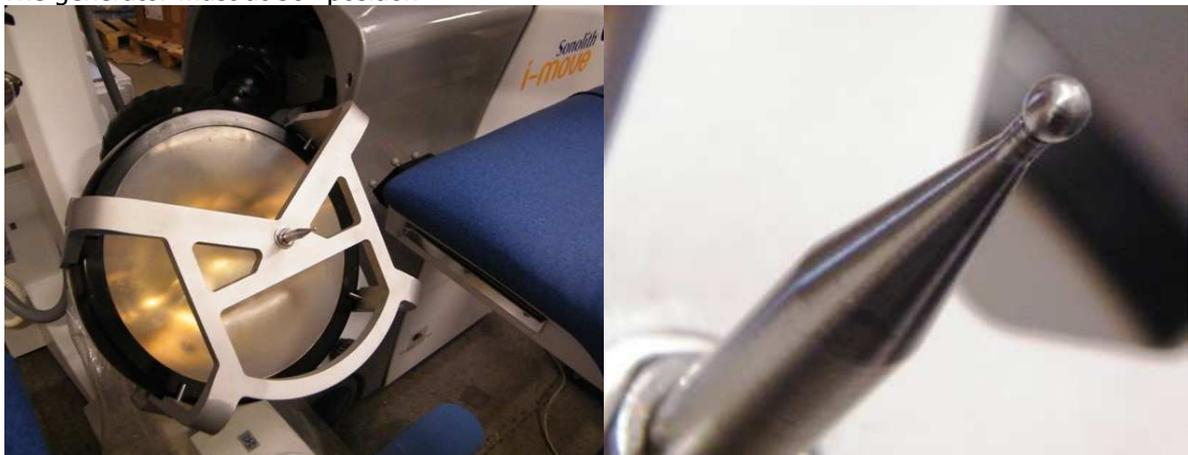
Figure 15 : F2 calibration tool in position for X-ray calibration
