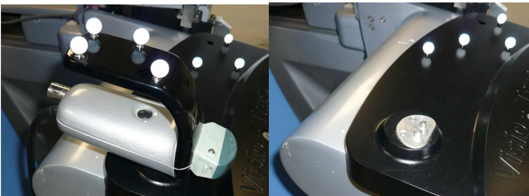
Figure 3: Calibration check of the Visio Track
