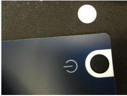
1. Remove the protective film from the back of the new lexan.
