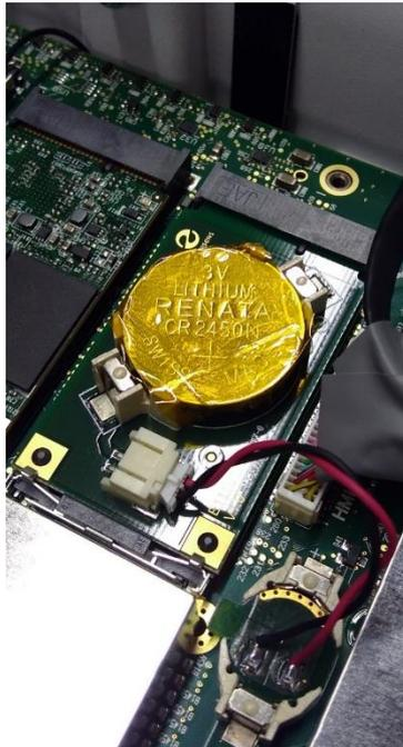
Place a string of Silicon type LOCTITE AS1701 along the MSATA holder.
