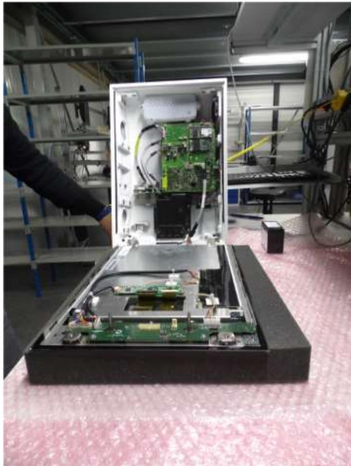
In order to exchange the following cables just cut the strip and disconnect both sides of the cable
