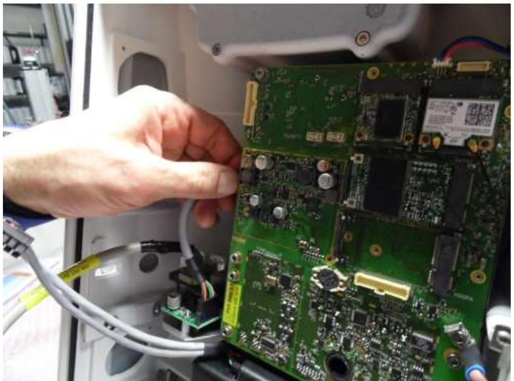
In order to remove the WIFI/Bluetooth PCB with the help of a clamp disconnect both antennas and bend the spring to lift up and slide out the PCB.
