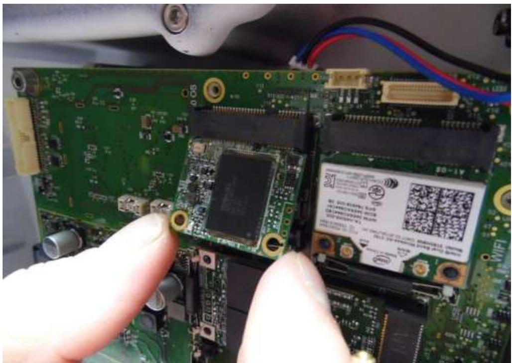
In order to remove PV3 module, unscrew the 5 screws holding it to the chassis (including the screw deep in the black plastic hole)
