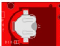
**Figure 17: Backup Battery Compartment**
