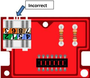
When an L-Net Termination T-Tap is wired onto an L-Net cable via a transposed color code label, the signals in the 'green' pair will be shorted together and the signals in the 'orange' pair will be shorted together. This will immediately disrupt communication for all devices that share the affected L-Net cable. This fault would be noticed immediately upon application of power to the devices connected to the L-Net cable.
