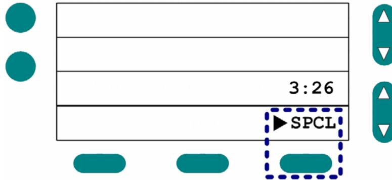
Figure 58: Special Mode Softkey with Activity Indicator
