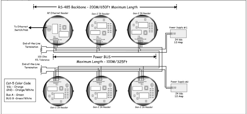
The RF Reader (Bus Master) may be connected at any location on Bus. Both ends of the RS-485 Backbone require end-of-the-line termination. **Recommended Cable Type:** CAT5 Stranded (4x2x26AWG)
