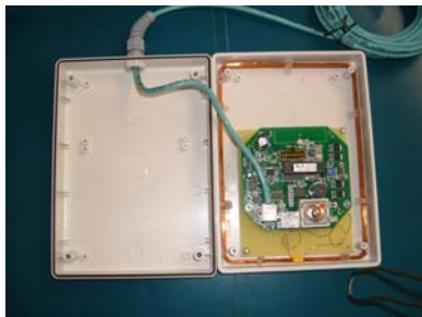
Figure 7-2. RF RDR With Cover Open
