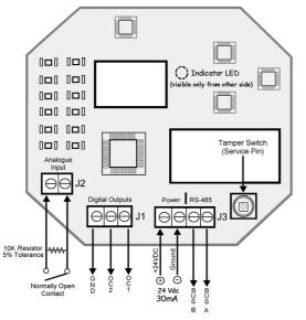
The reader also has a Service Pin/Tamper Switch 'that generates service messages when pressed to aide device registration. The switch also indicates attempts to remove the device's cover after the device is registered.
