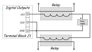
Recommended Cable: 22 AWG, unshielded/twisted pair, Max Distance: 1,000ft/300m
