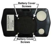
2. Separate the battery cover from the back of the badge by inserting a small screw driver into either of the square slots adjacent to the battery cover. Gently lever the screw driver outwards until the battery cover releases from the badge.
