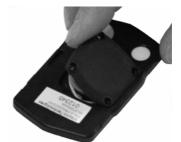
6. Once the battery cover is in place, tighten its 4 screws into place.
