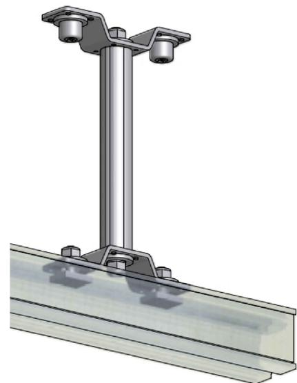
DETALLE ANCLAJE A LOSA
