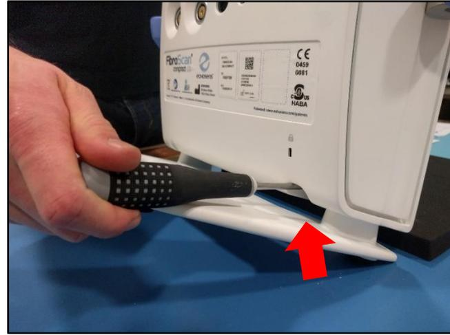
Push with a screwdriver the screw on the right on the back of the device.
