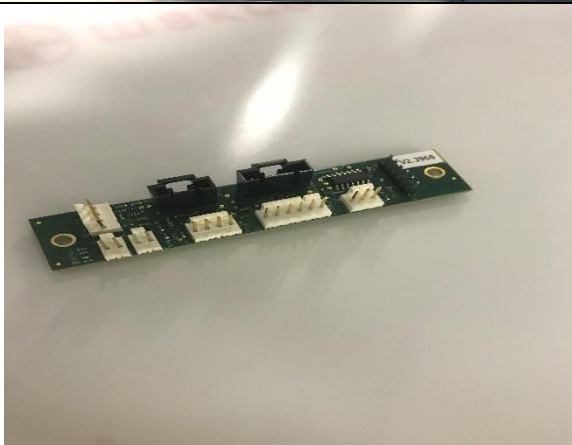
M200143 Remote Controller board 502T1
